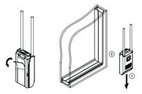
6 Remove the protective film from the cord tensioner, and with the cord under slight tension stick the cord tensioner to the glass. CAUTION! When adjusting the blind, please move the cord only parallel to the glass.
