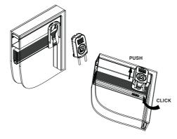
3 Slide the magnetic housing unit into the self-centring base plate, pushing the former upwards until it is correctly locked, as confirmed by the click of the "Push" button.
