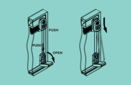
Removal of external magnetic device from glass
